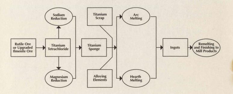
Process Flow Chart of Titanium Production reprinted with permission of RMI Company, Niles, Ohio
